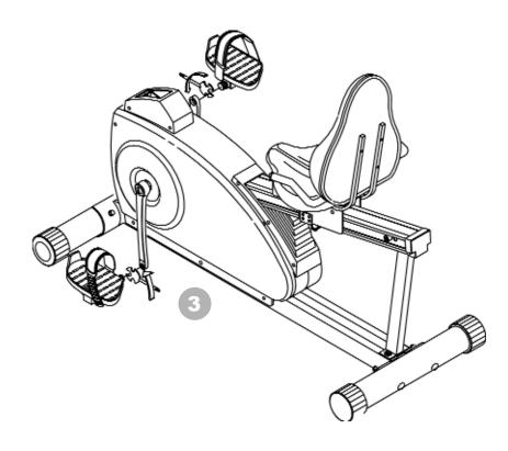
**3.** Attach pedals (30, 31). Axles of pedals are branded "L" and "R." The pedal marked "R" goes on the right hand side of the bike and the one marked "L" on the left hand side. Tighten the left pedal by turning counter-clockwise and the right pedal by turning clockwise.
